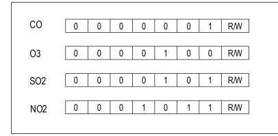
The R/W bit is also used as a common data bit. When reading/writing, use 1 or 0 perform 'OR' operation with original data (read as 1, write as 0). See the figure below for details.
